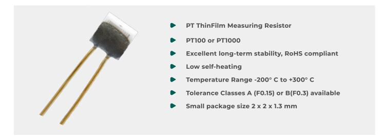
Variohm ERTD2 series ThinFilm Platinum Elements are durable and designed for applications where long term stability, interchangeability and accuracy over a large temperature range are important. Applications include automotive, white goods, HVACR, energy management, medical and industrial.
